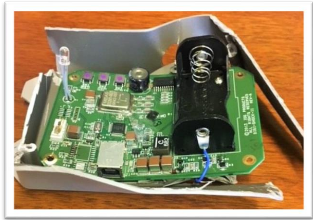
Device case damaged showing bent circuit board. Battery case cracked broken.
