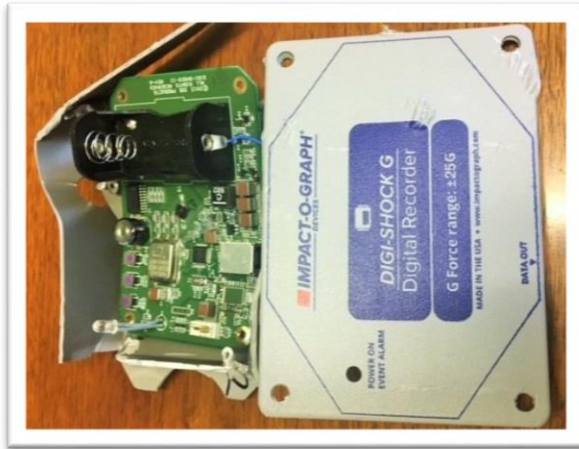
Digi Shock G cover (little damage) but case and circuit board extensive damage
