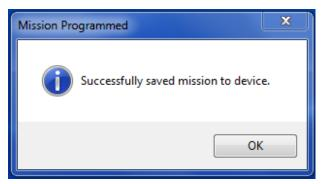
After programming a mission the device will perform a self check and calibration. This will be evident by about 35 seconds of continuous LED blinking. It will then give a single bright flash.
