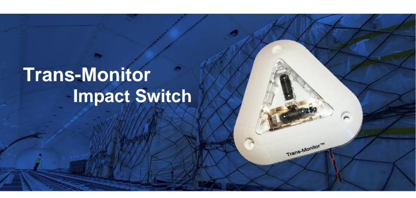
The Trans-Monitor Impact Switch (TMIS) consists of two sets of spring loaded steel balls that hold copper contacts apart, creating an open circuit through the device. If impacts are greater than the G force of the device, the balls will dislodge from their set positions completing the circuit from the connected wires of the device installed to your eternal circuit. Depending on the configuration of your external circuit, the TMIS will either turn on or turn off your equipment.
